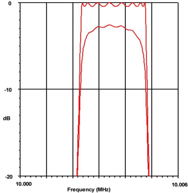
The top graph shows the frequency response of a filter made of perfect, loss-free, crystals while the lower response shows the result of incorporating typical real-world crystals having a Q of 100,000. Even such high quality crystals have sufficient loss to cause the rounding of the edges of the pass band in the prototype filter shown in the previous diagram.
