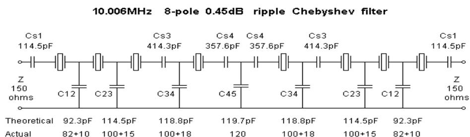
This is the circuit of the 8-pole filter showing calculated values for the capacitors. Also shown are the nearest standard values which were actually used for the coupling capacitors. These were selected from stock using a capacitance bridge. It was found to be easy to select pairs of capacitors within 1-2pF of the desired value.
