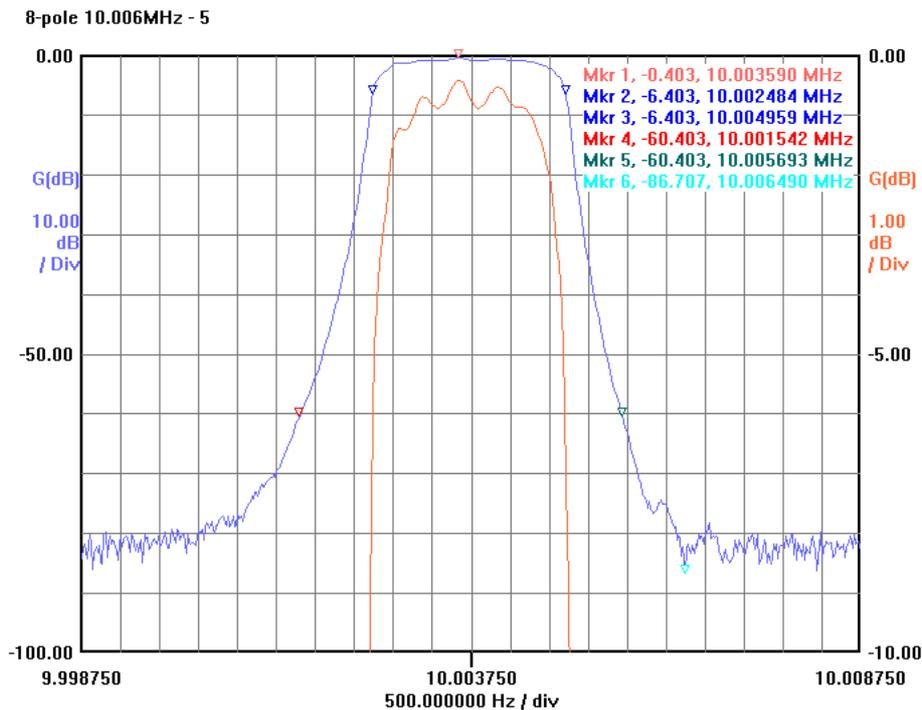
The markers show that the bandwidth is 2475hz at -6dB, and 4151hz at -60dB; thus the 6:60 dB ratio is 1.7:1 . The stop band rejection is better than 80dB, but see later how I improved this figure to more than 90dB. Also included here is an expanded trace of the pass band. This shows that while the ripple is very close to the design specification of 0.45dB there is an unavoidable droop at each side of the pass band which is due to the finite Q of the crystals.
